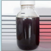
Turbine oil BEFORE filtration with the VRU
