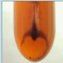
Ultra Centrifuge test, initial sample before the VRU (inlet)
